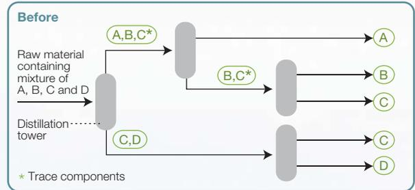
Reviewed process of distilling twice to extract component A, reducing energy used in distillation by distilling once
