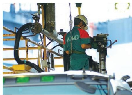
Filling a tank truck with a safety belt
