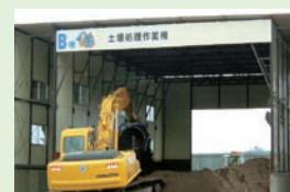
Sorting the soil at an intermediate treatment facility
