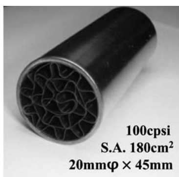
図2 Metal honeycomb substrate for the structured catalyst.
