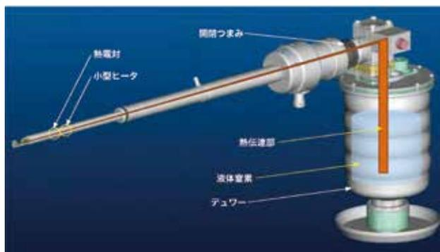
図3 冷却ホルダー<sup>2)</sup>
