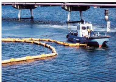
Extending oil fences and recovering oil in a drill to prevent seawater contamination
