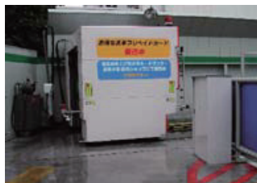
Car washing machine with water recycling function
