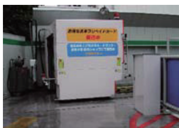
Car washing machine with water recycling function
