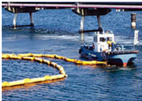
Extending an oil fence as part of a drill to stop marine pollution
