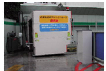
Car washing machine with water recycling function
