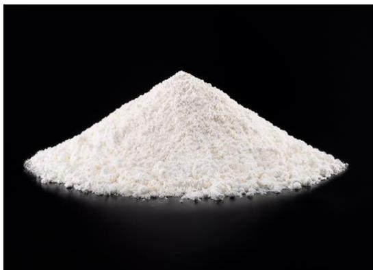
XYDAR® LF-31P Low-Dielectric Liquid Crystal Powder (LCP)
