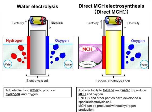
(Reference) Overview of "(2) Direct MCH electrosynthesis" (comparison with water electrolysis)
