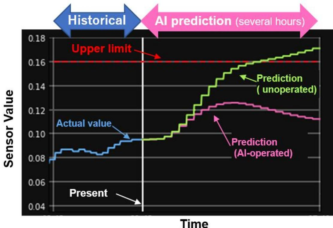
The AI system had predicted that the sensor value would exceed the upper limit if unoperated (green); the system automatically operated the control element to keep the value within the prescribed range (pink).
