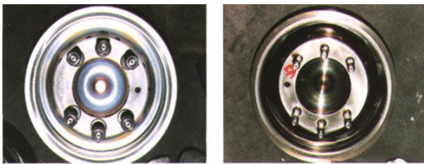
Left side: Under crown after 8000 h (SL SERIES)
