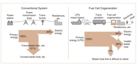
A model comparing the energy efficiency of the previous system and the decentralized system.
