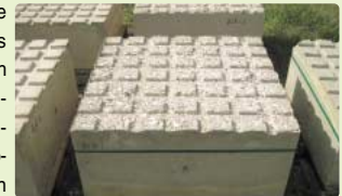
Algal reef made from oyster shell, which is used as aggregate
