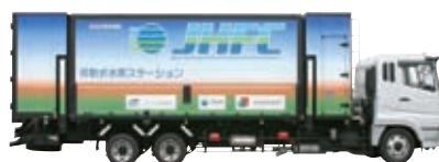
Mobile hydrogen refueling station
