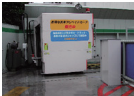
Car washing machine with water recycling function
