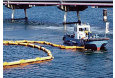
Extending an oil fence as part of a drill to stop marine pollution
