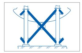
\* Parts used for cross bracing, which reinforces steel frames, are erected at the base of spherical tanks to enhance their safety.
